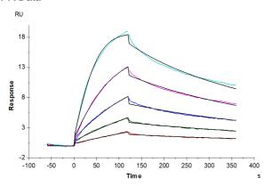
Human EGFR, His Tag captured on CM5 Chip via anti-his antibody can bind Human EGF, hFc Tag with an affinity constant of 0.39 nM as determined in SPR assay (Biacore T200).
