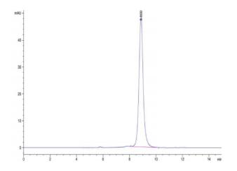
The purity of Human EGF is greater than 95% as determined by SEC-HPLC.
